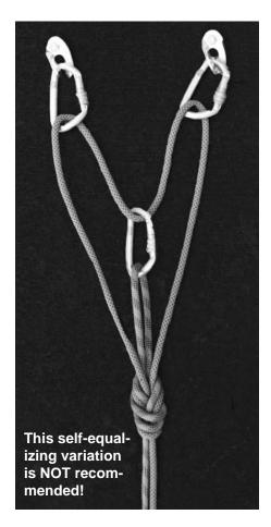
has been shown to work poorly at distributing the load. Not only that, it can be downright dangerous in the event of a failure of any single item of gear in the rigging!
