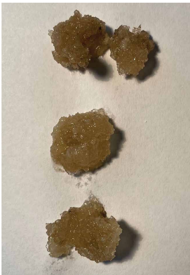
Figure 8. Globular thenardite/blodite precipitates, 2-3 cm diam.
