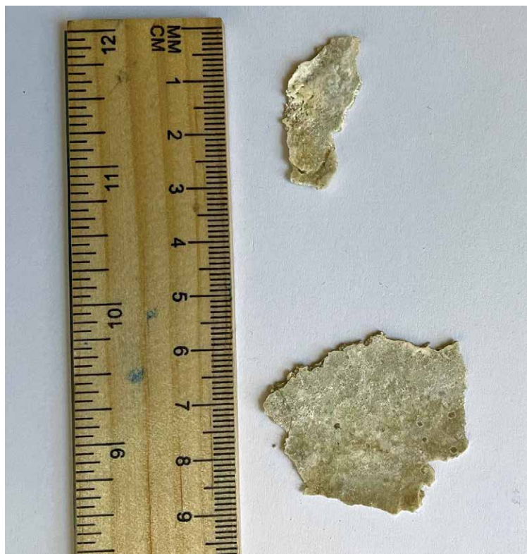
Figure 18. Simulated crust from evaporated cave stream water.
