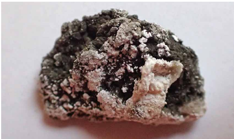
Figure 16. Sulfate coating on damp shale, 3cm diam.
