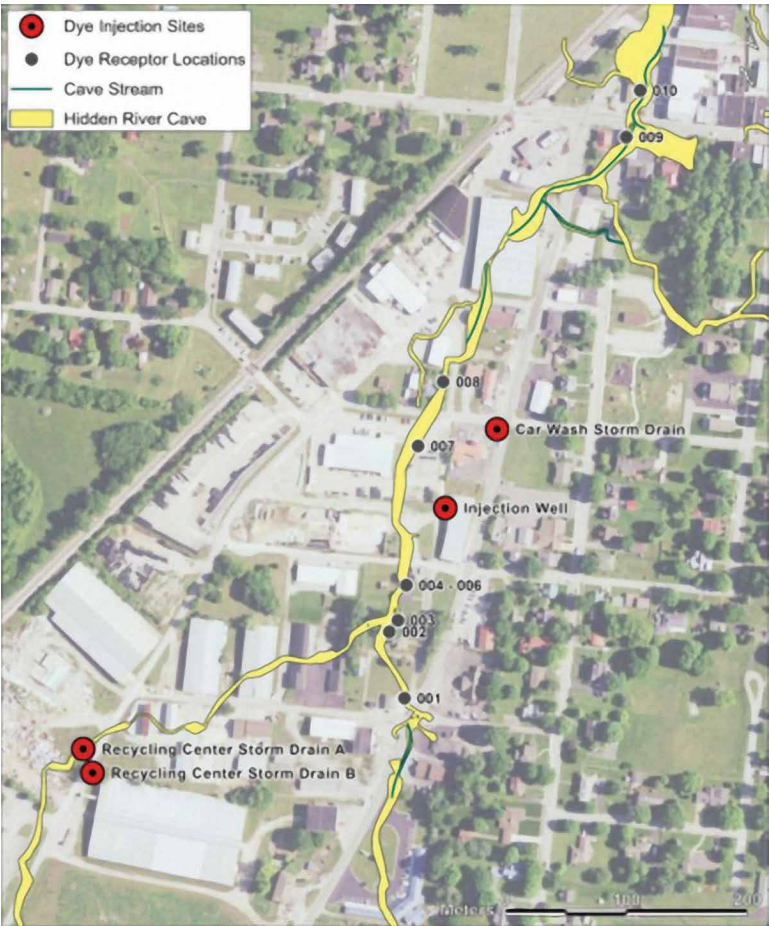
Figure 5. Dye receptor sites in Hidden River Cave and dye injection locations in Horse Cave. Data from the CRF and the KGS.
