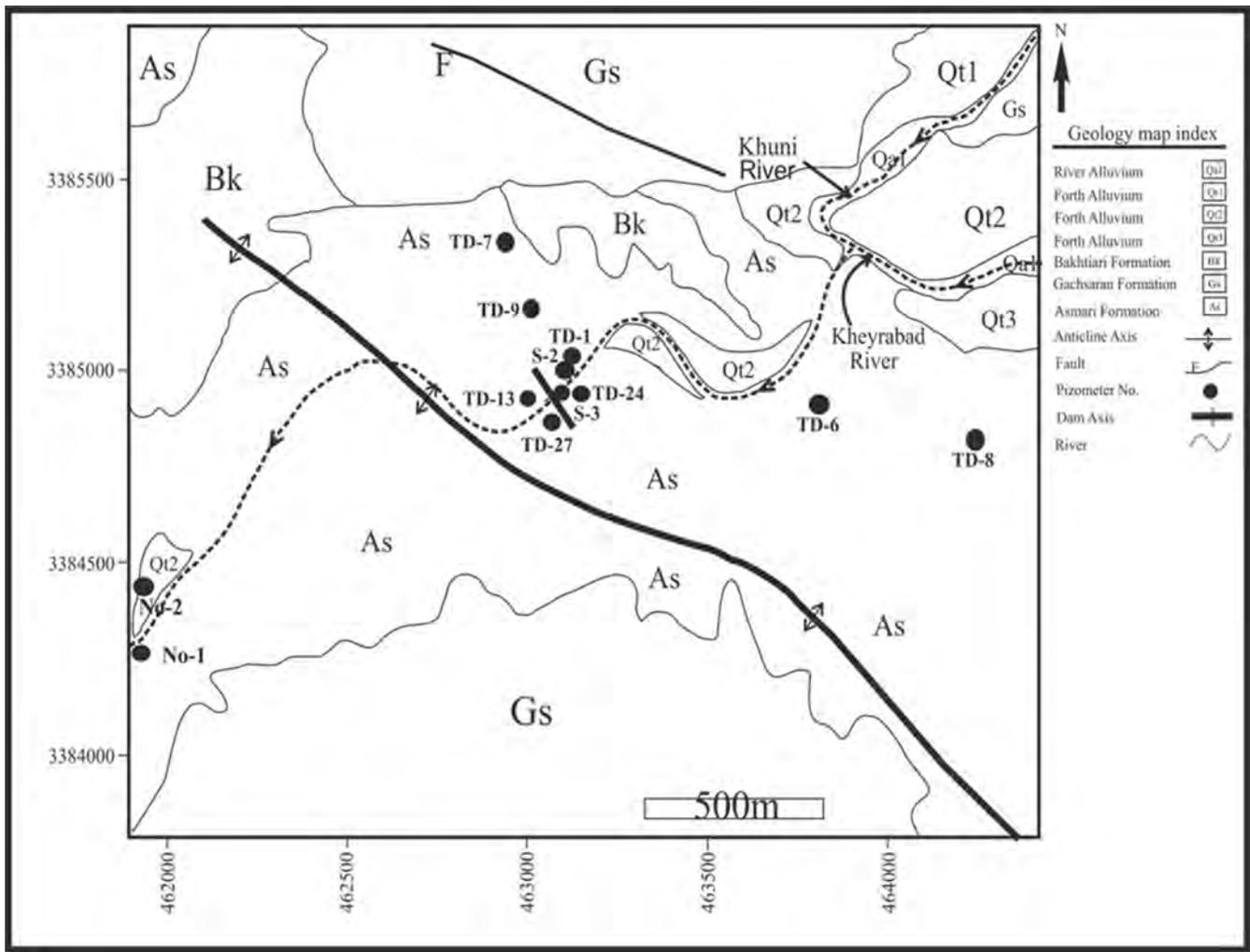
Figure 10a. Geology map of Kowsar Dam Site and boreholes.
