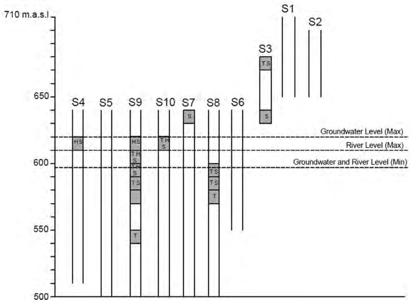
Figure 8b. Fluctuation of groundwater level and river level at boreholes in Symareh Dam Site.
