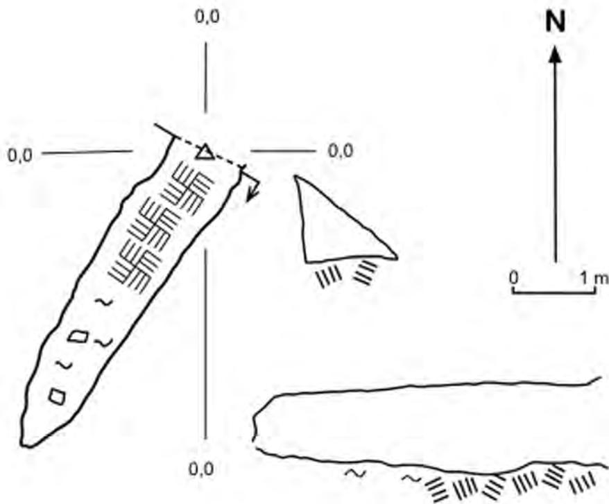
Figure 2. Survey of Główniowa Nyża Cave showing a corridor of the cave throughout the length of the cave profile; reproduced from Zwijacz-Kozica (2011). The symbols: four lines all labeled 0.0 are indicating entrance to the cave (origin of the local coordinate system); 3 sketches show: 1 – cave profile, 2 (small triangle) - cross section of the cave entrance (direction indicated by arrow on the cave), 3 - cross section of whole cave; soil - clusters of parallel lines.
