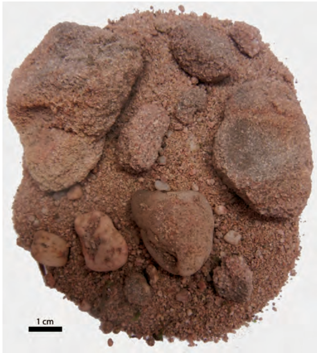
Figure 11. LMRC-1 collected from collapse boulder in sinkhole. Note iron oxide staining.
