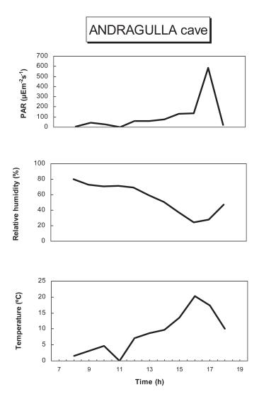
Figure 4. Photosynthetically active radiation (PAR), temperature, and relative humidity from sunrise to sunset in Andragulla cave at a cyanobacterial mat of *Scytonema mirabile* and *Gloeocapsa sanguinea*.
