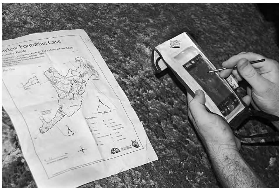
Figure 5. The PDA device was protected in the field with an Aqua Quest, water-proof cover.
