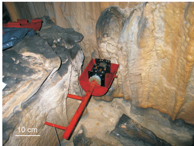
Figure 3. Monitoring site Postojna 1 with TM 71 instrument (photo S. Šebela).
