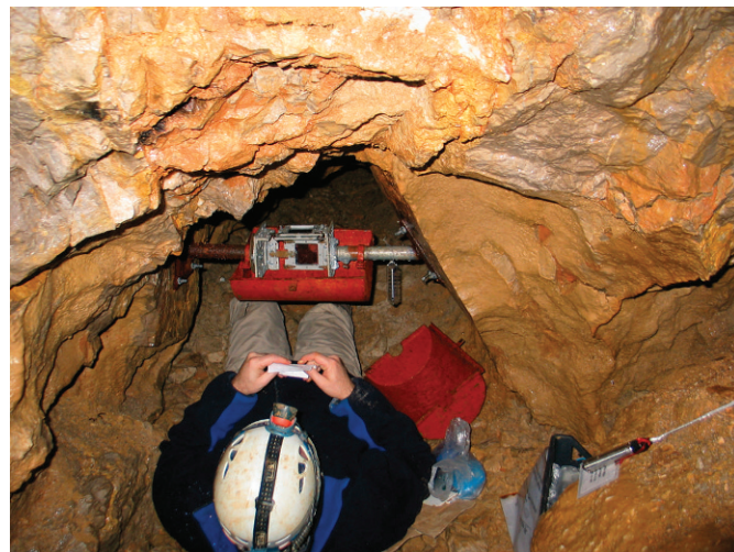
Figure 4. Monitoring site Postojna 2 with TM 71 instrument (photo S. Šebela).
