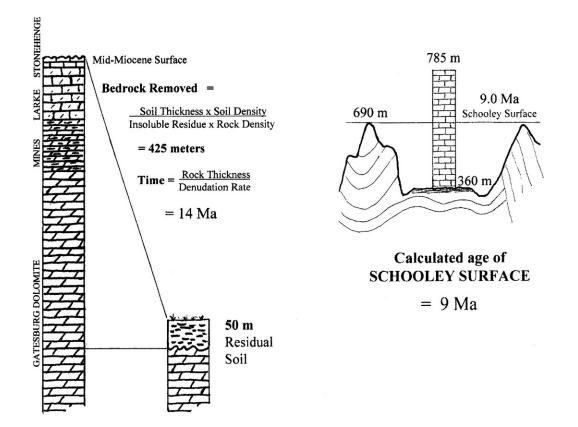
Figure 3. Carbonate rock denudation in the Nittany Valley, Pennsylvania. Estimation of thickness of removed carbonate rock from residual soil taken from Parizek and White (1985).
