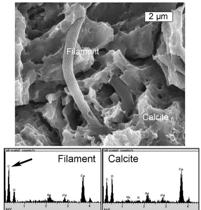
**Figure 6.** Scanning electron micrograph of reticulated filament and two EDX analyses; one centered on the filament and one centered on the calcite next to the filament. The analyses extend 2–3 µm into the sample so both plots show calcite (Ca + C + O), trace amounts of clays (Mg + Si + O) and the gold-palladium coating medium (Au + Pd). Note that the filament contains more carbon than the calcite sample indicating that the filament itself is carbon-rich.
