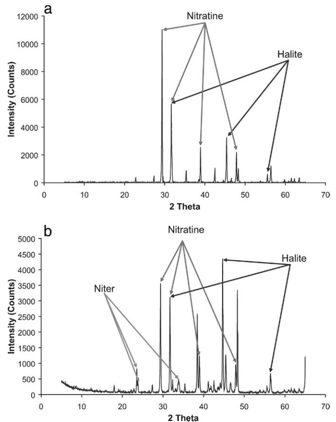
**Figure 3. X-ray diffraction (XRD) data. Patterns were generated using Cu K- $\alpha$  radiation. (a) Example of XRD pattern from the cemented level showing the presence of nitratine (peaks marked) (b) XRD pattern of nitratine from the University of Texas collection (peaks marked).**
