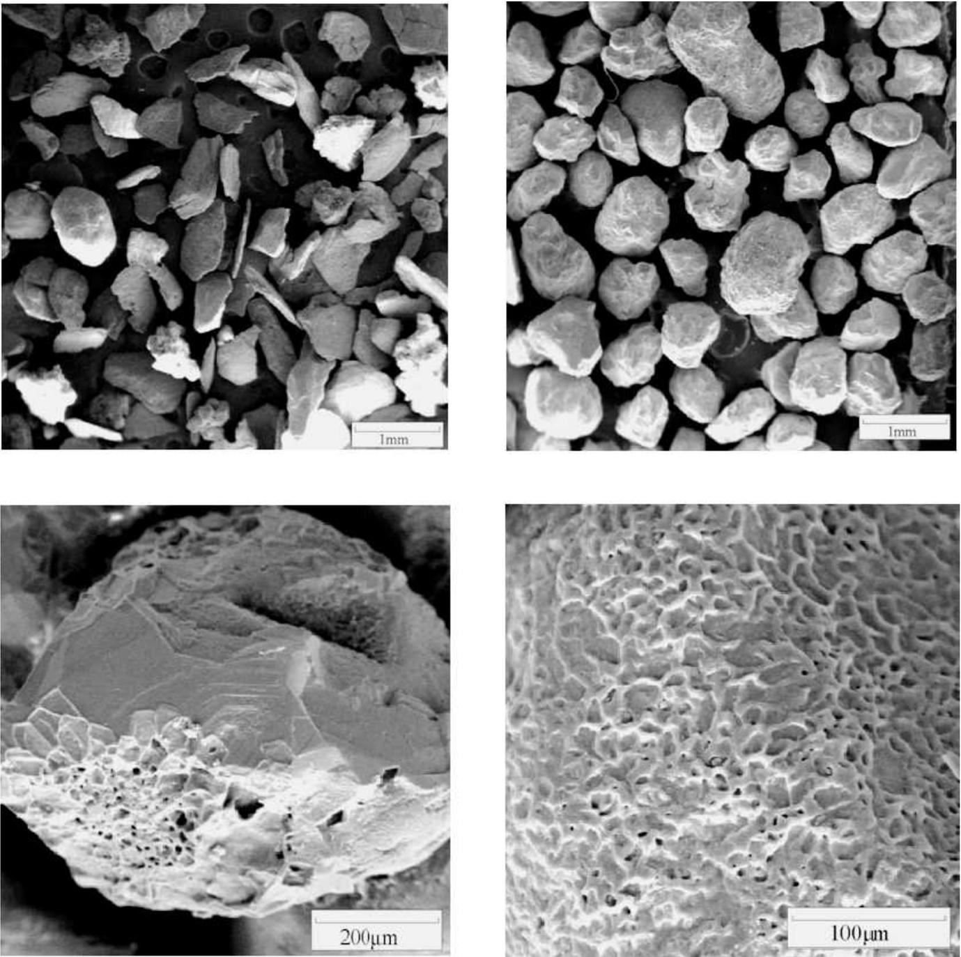
**Figure 12.** Surface of quartz grains. Top left – mixture of quartz and angular grains from Bed 3 in Section 1; top right – quartz from modern soil; bottom left – a detail of quartz corrosion from Bed 15 in Section 1; bottom right – a detail of newly-formed quartz precipitates from Bed 2 in Section 2A.
