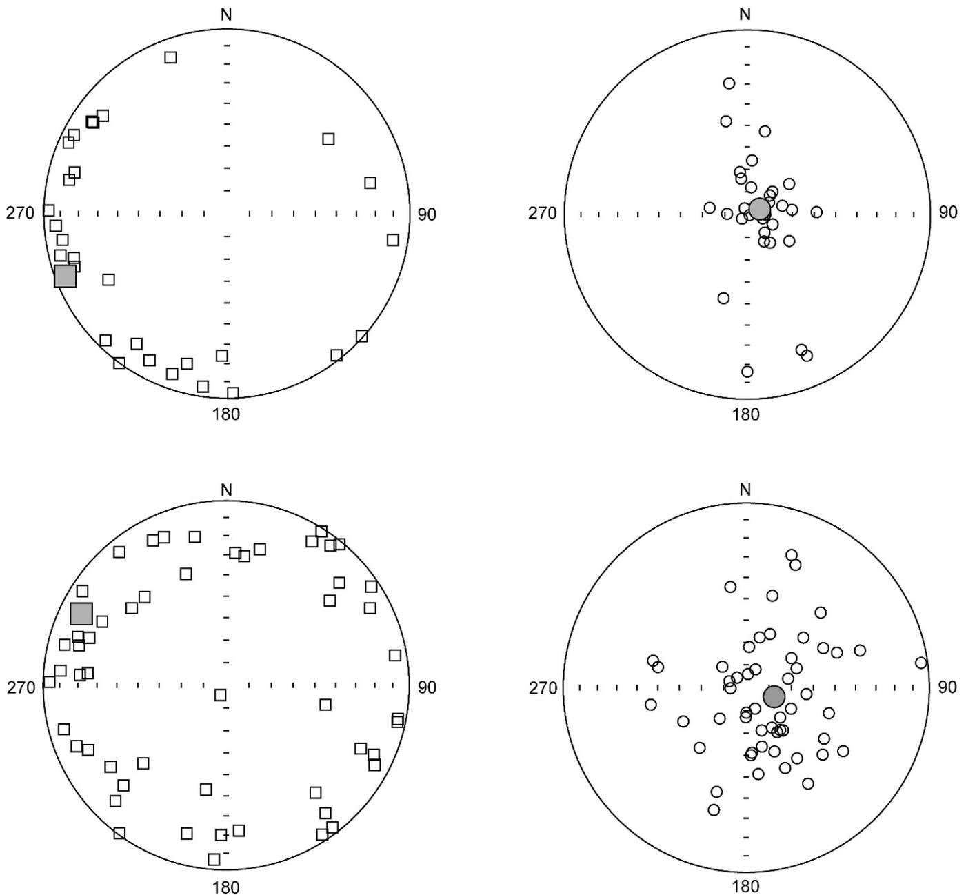
**Figure 10.** Principal directions of magnetic fabric of sediments indicated by anisotropy of magnetic susceptibility; equal-area projection on the lower hemisphere. Top left – magnetic lineation in bottom sedimentary beds; top right – pole to magnetic foliation in bottom sedimentary beds; bottom left – magnetic lineation in top sedimentary beds; bottom right – poles to magnetic foliation in bottom sedimentary beds; larger gray squares and circles represents mean directions.
