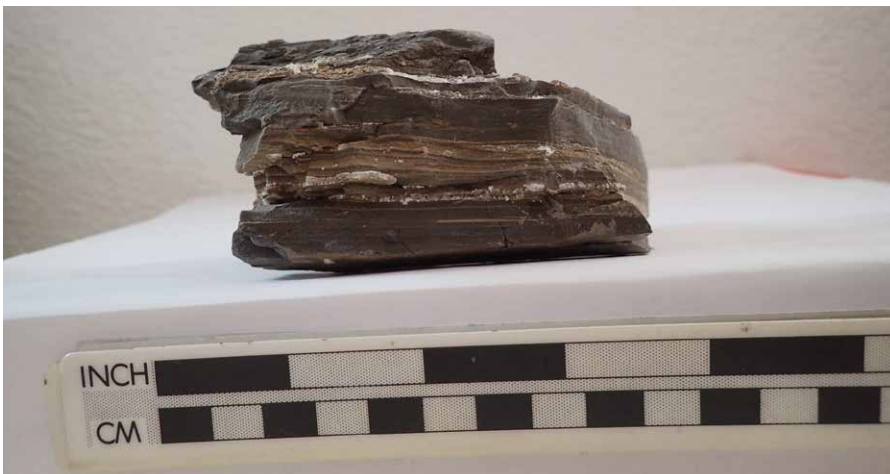
Figure 15. Shale containing gypsum fracture fillings and goethite laminations.
