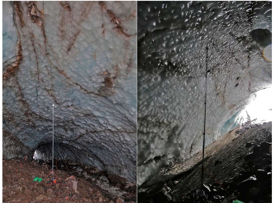
Figure 17. Location of the ultrasonic anemometers in Hot Imagination Cave. View out of the cave in upper picture, view inside cave in lower picture.
