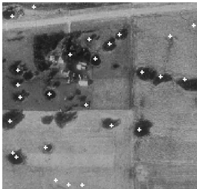
Figure 14. Verified and adjusted sinkhole locations on a DOQ in an area of Wykoff Quadrangle, Fillmore County using Location-Verification and Spatial Transformation tools in ArcView GIS. (A) sinkhole locations before spatial transformation. (B) sinkhole locations after spatial transformation. The cross on the aerial photo reflects sinkhole locations on the land surface.
