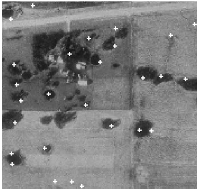
Figure 14. Verified and adjusted sinkhole locations on a DOQ in an area of Wykoff Quadrangle, Fillmore County using Location-Verification and Spatial Transformation tools in ArcView GIS. (A) sinkhole locations before spatial transformation. (B) sinkhole locations after spatial transformation. The cross on the aerial photo reflects sinkhole locations on the land surface.
