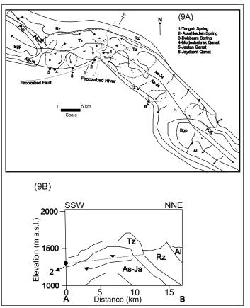
Figure 9. Hydrogeologic maps and regional flow pattern (A) and geologic cross sections (B) of Podenow Anticline. Legend is referenced in Figure 5.
