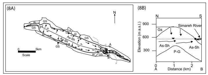
Figure 8. Hydrogeological maps and regional flow pattern (A) and geological cross sections (B) of Ravandi Anticline. Legend is referenced in Figure 5.
