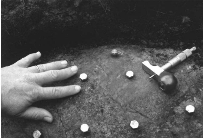
Figure 2. The Rock Erosion Meter at measuring site #95-29. The instrument can be slipped into six different measuring positions for each bolt. By rotating the large knurled handle, the measuring rod moves in and out. Photo by C. Allred.
