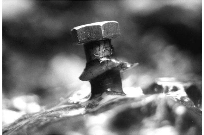
Figure 11. Soon to fall out, station 94-23 is increasingly exposed by highly acidic muskeg drainage over the limestone. The apron of overflowed epoxy is at the former level of the rock surface.
