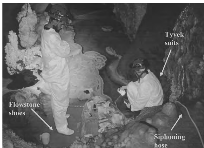
Figure 3. Biofilm sampled from water siphoning hose at Red Lakes Pool located in the Western Branch of Lechuguilla Cave. This figure also demonstrates flowstone shoes, Tyvek suits, and other sterile techniques used during sampling. Andy DuFrane left, Andrea Hunter right. Photo by Val Hildreth-Werker.
