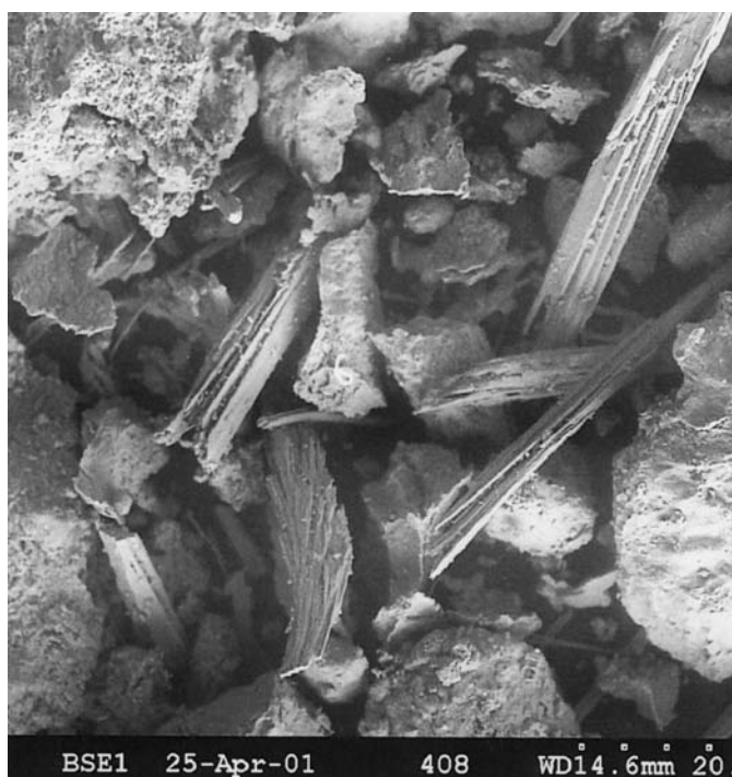
Figure 10. Scanning electron microscope images of rock flour. (A-top) Sample 402 from Turner Avenue consists mainly of etched calcite rhombs. (B-bottom) Sample 408 from Turner Avenue at intersection of Dead Bat Trail is a mix of limestone rock fragments (large lump), acicular gypsum crystals, and some minor quartz sand grains.
