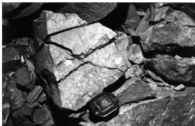
Figure 5. Massive bedrock shattered by growth of gypsum in fractures producing Type I breakdown. Brunton compass provides scale.
