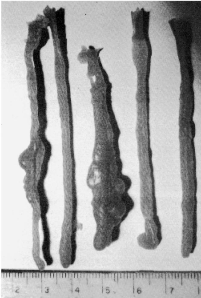
**Figure 12. Some tubular paraffin stalactites. The scale is in centimeters. Photo by C. Allred.**
