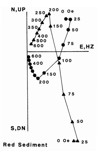
Figure 4. Demagnetization diagram showing primary and secondary components of magnetization. Dots indicate magnetic declination plotted in N, E, S (north, east, south) coordinates. Triangles represent magnetic inclination plotted in UP, DN, HZ (up, down, horizontal) coordinates. Numbers show alternating field demagnetization intensity in Oersteds (Oe). Note that the normal secondary component is removed by 200 Oe demagnetization step.
