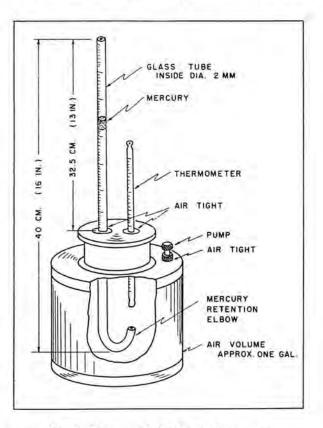
Fig. 1. Diagram of the Speleo-Barometer.
