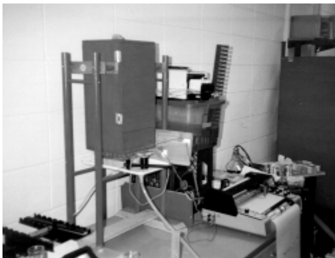
Figure 5. Photograph of the experimental apparatus showing the recharge water delivery system and the syringe pump used to introduce the tracer.
