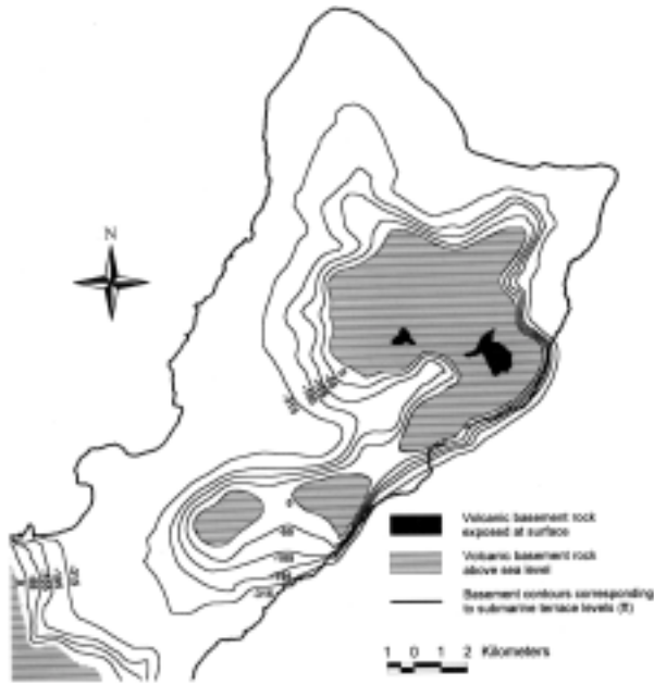
Figure 4. Contours (in feet) on volcanic basement rock corresponding to modern sea level and the four submerged terrace levels as mapped by Emery (1962).
