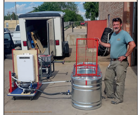
Knutt Petersen shows the hinged cover of the 2 x 6 foot decon tank. The black tubing recirculates the hot water through the propane heater and sends it back with a thermal boost through the white tube.
