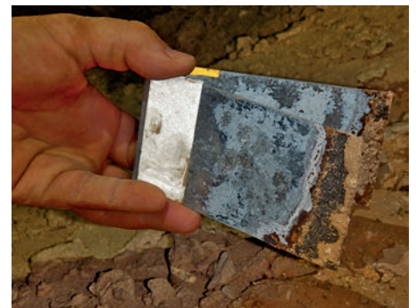
Galvanized steel signs altered by corrosion
